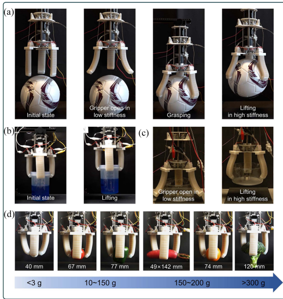
Fig. 9. HVS structure enhanced grasping capability of the soft gripper. (a) Grasping of a football (diameter \sim 19.0 cm, weight \sim 340 g). (b) Grasping of a cup of water ( \sim 650 g). (c) Grasping of a glass tank ( \sim 15.1 cm, \sim 400 g). (d) Grasping of various fragile objects with shapes ranging from 40 mm to 120 mm, and weight ranging from 2.7 g to 300 g.
